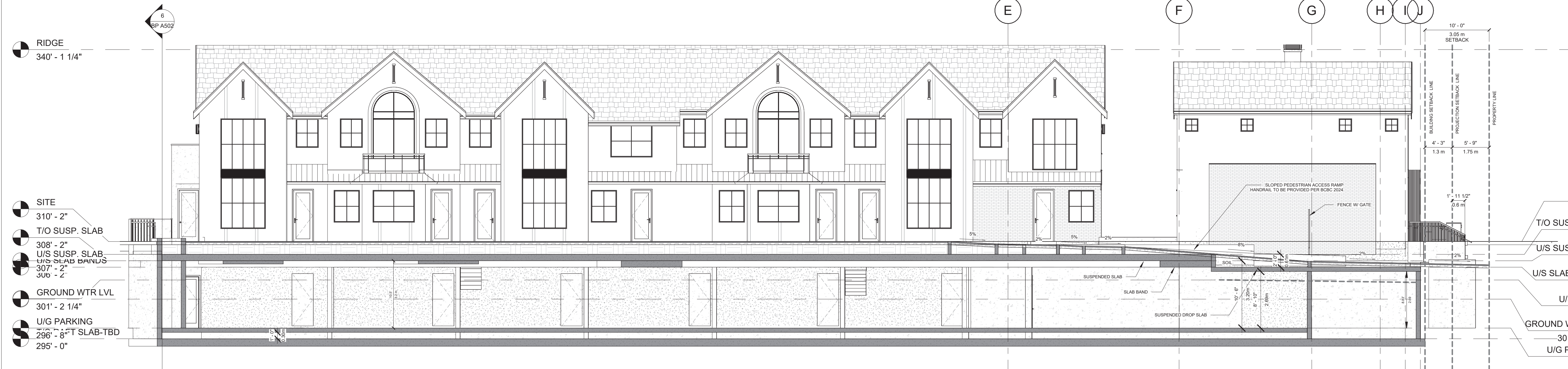
1 BP SECTION PARKING ENTRY RAMP 1/8" = 1'-0"
