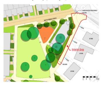
This interim scenario provides a 4 metre wide vehicle/pedestrian shared-use path for the residences. One meter width of the shrub planting along the path, and the northeast corner of the planting bed would be affected by the access.
