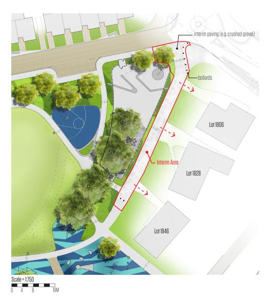
This interim scenario provides a 4 meter wide vehicle/pedestrian shared-use gravel path for the residences protected by fixed and removable bollards. The slope in the planting area on the northeast corner of the dog park will be implemented for the ultimate scenario to be achieved. A portion of the dog park fence will also need to be adjusted along with additional tree planting as per the Preferred Ultimate Concept Design.
