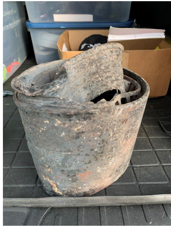
Figure 16. Other L1 bearing components post recovery.
