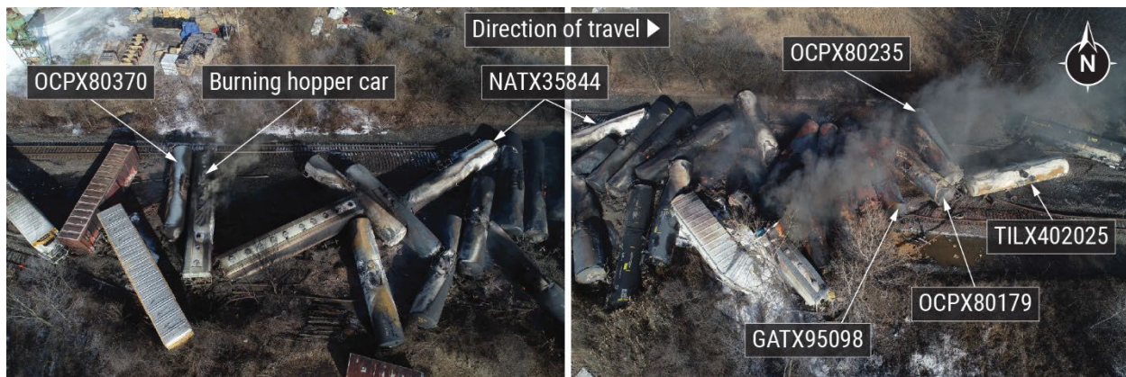
Figure 7. Derailment pileup and VCM tank cars.
