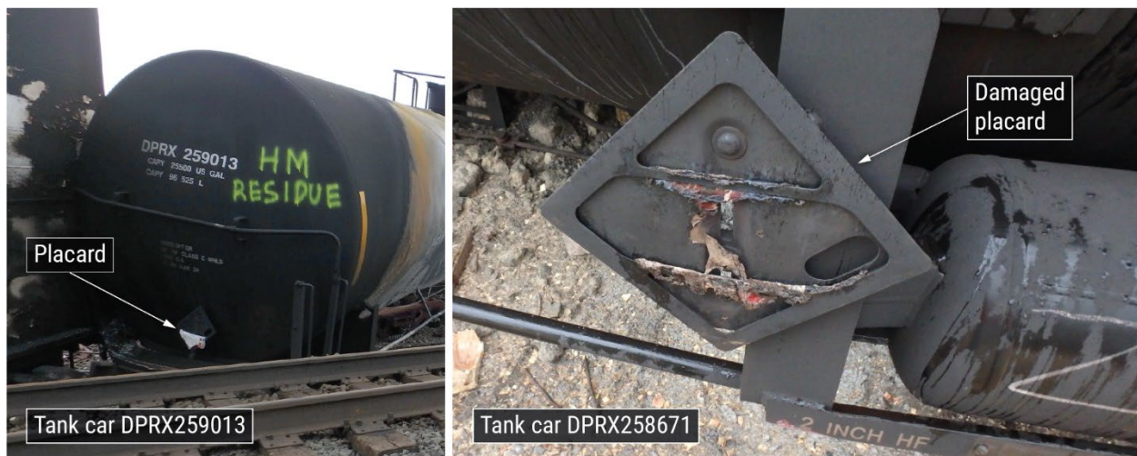
Figure 26. Postderailment photographs of placards exposed to heat.
