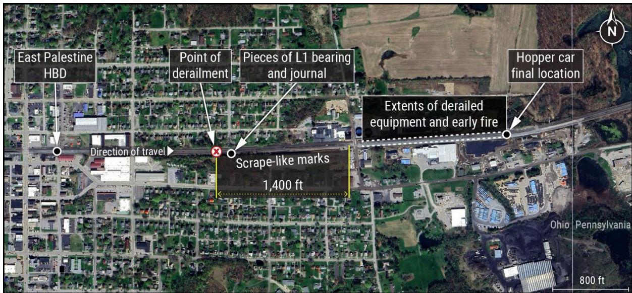
Figure 28. Locations of derailment evidence.
