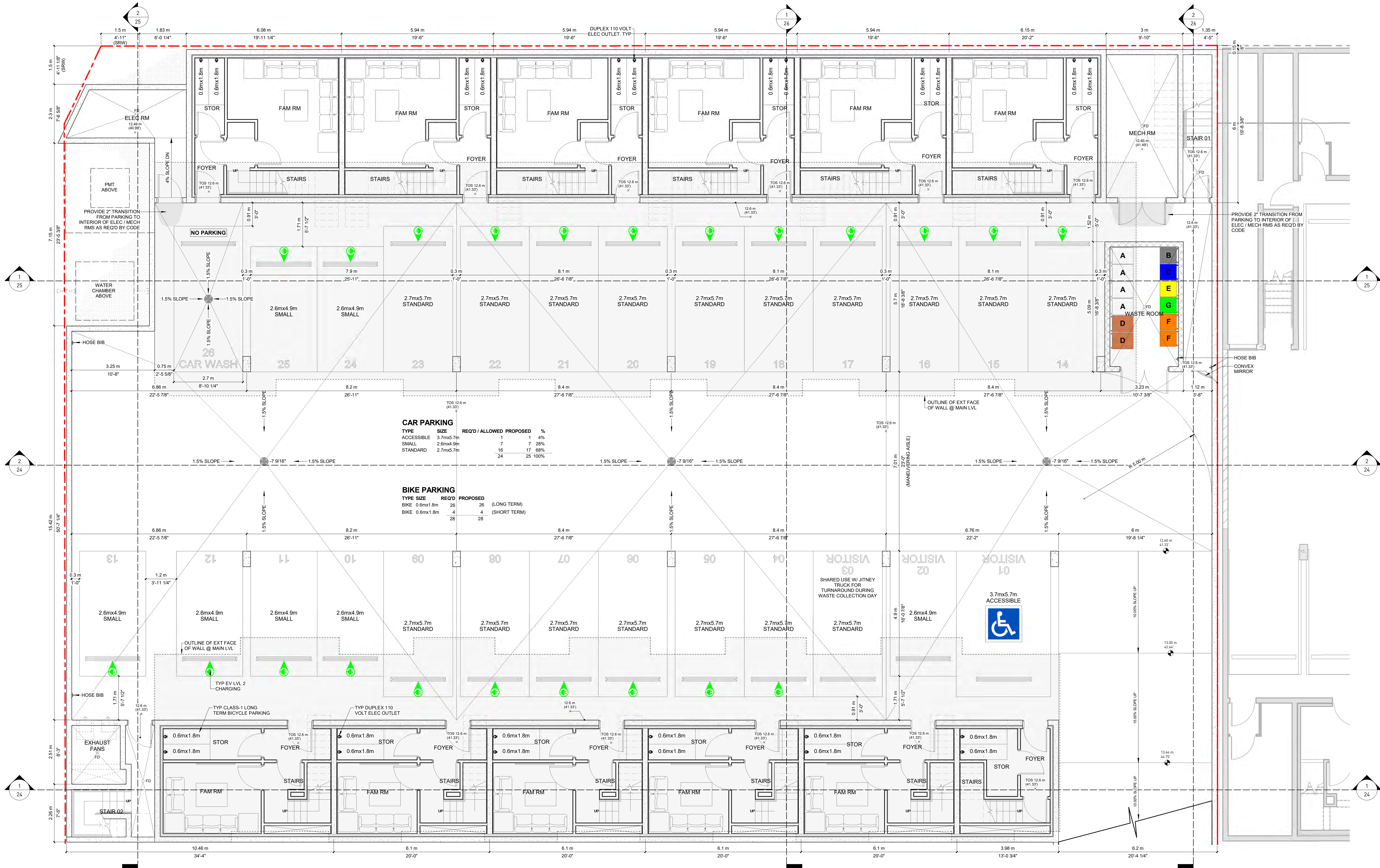
1 PARKADE LEVEL FLOOR PLAN 3/16" = 1'-0"
